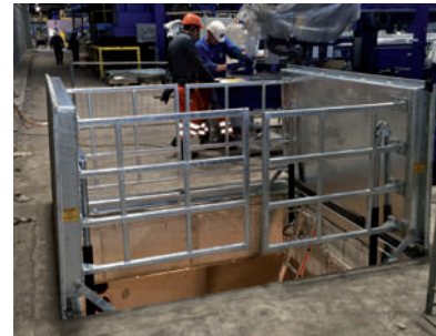
Hydraulic shaft cover as an assembly opening with anti-fall-in protection that can be driven on with a forklift truck – Krefeld
