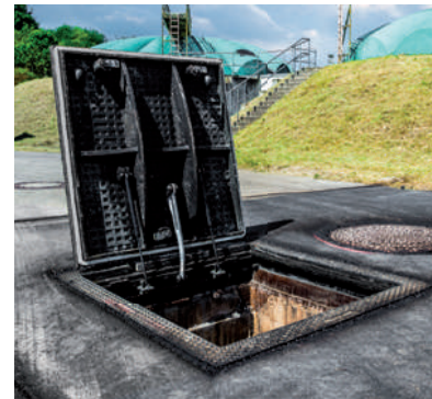
Surface-water-tight cast-iron cover with an opening aid, a load class of D400 and a clear opening of 1000 mm x 1000 mm – Munich
