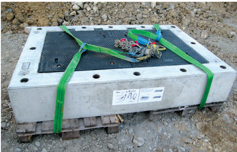
Prefabricated surface-water-tight cable shaft cover with a height-adjustable reinforced concrete frame and a load class of D400 – Biel, Switzerland
