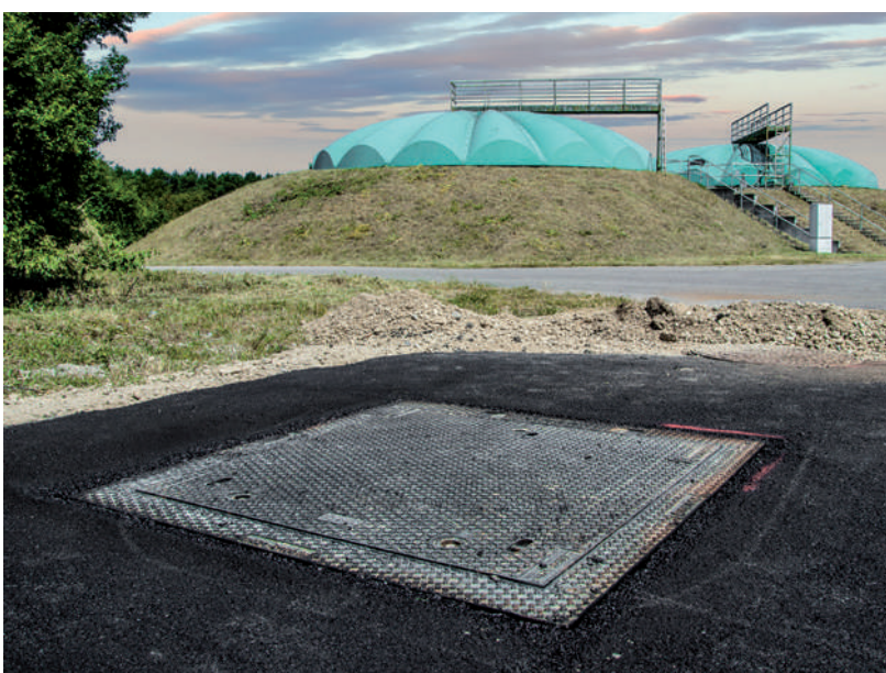
Surface-water-tight cast-iron cover with an opening aid, a load class of D400 and a clear opening of 1000 mm x 1000 mm – Munich
